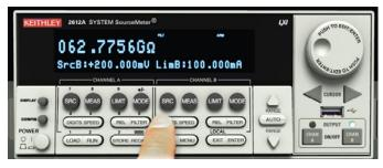
Figure 5. Adjusting an SMU instrument's resolution.
